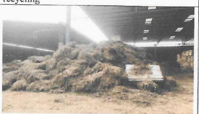
Photo 8: Fuel (cane silts) for boiler
